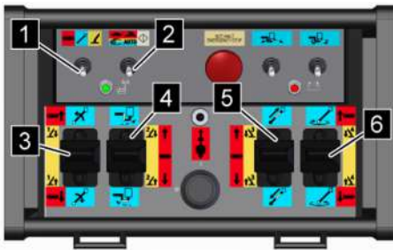
Fig. 94: Operation of outriggers
