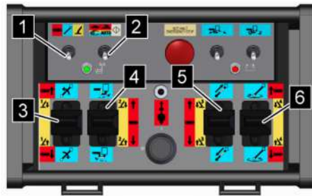
Fig. 89: Operation of outriggers
