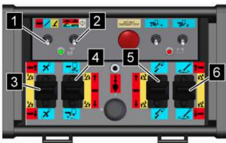
Fig. 96: Operation of outriggers
