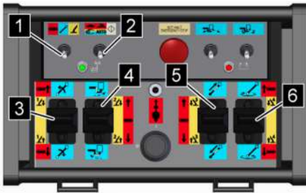
Fig. 87: Operation of outriggers
