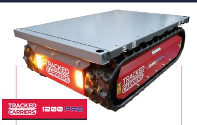
The 1200 series from Tracked Carriers is the ideal all-round carrier. At just 750mm wide the 1200 R and 1200 PRO models can fit through most doorways, and with a substantial 1,200kg maximum capacity the uses are endless.
