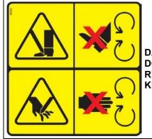
DANGER - MOVING BLADES. DO NOT REMOVE SAFETY GUARDS WHILST ENGINE IS RUNNING. **KEEP HANDS & FEET AWAY.**
