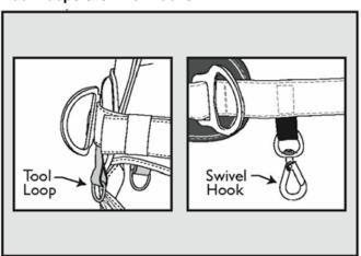
Loops and swivel hooks are fitted to some waist belts and are intended for use as attachment points for light tools or communication equipment. THESE LOOPS / SWIVEL HOOKS ARE NOT TO BE CONNECTED TO ANY LANYARD, RETRIEVAL SYSTEM, STRUCTURE OR PERSON.
