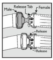
Connection of this buckle is a simple push fit. To release the buckle, both release tabs must be moved back simultaneously, if not, the buckle will remain connected. The mechanism MUST be kept clean at all times and you should NOT use any
