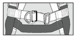
If the harness has a front fall arrest 'D' ring, it will be on the chest strap and the shoulder straps should be adjusted so that it sits on your sternum / breast bone.
