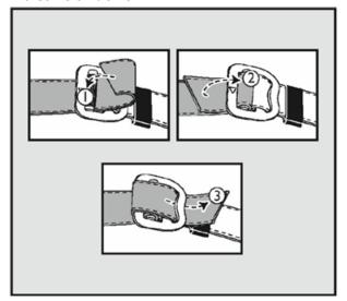
This buckle has to be threaded in a specific manner to ensure a secure fit. It is only fitted to harnesses that incorporate a Work Positioning Belt.
