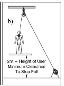
The anchorage for the G.Stop should be positioned so as to:
