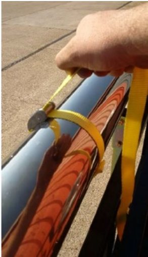
Securing the load using the lashing strap.
