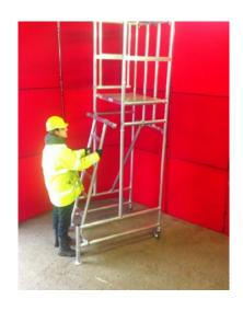
1) OPEN FRAME AND LOCK MECHANISM
